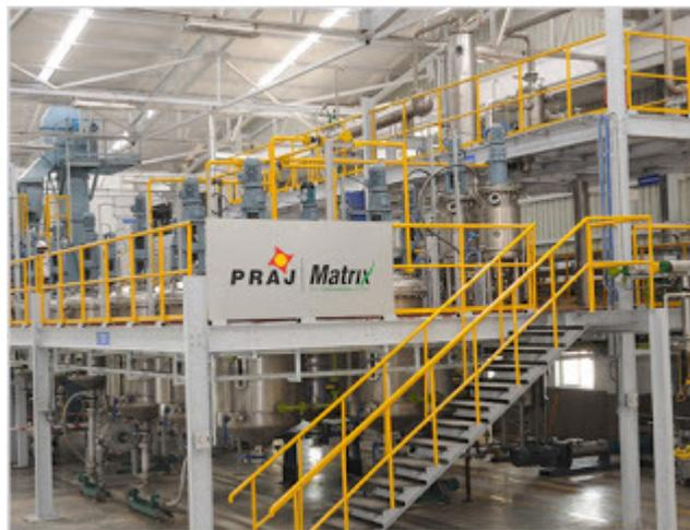
In its endeavour to create 2nd generation biofuels, the Praj Matrix Innovation Centre has set up a pilot plant for the conversion of lignocellulose to Bioethanol. Efforts to scale up this technology further will follow, and Praj hopes to be able to commercialise the technology in the
